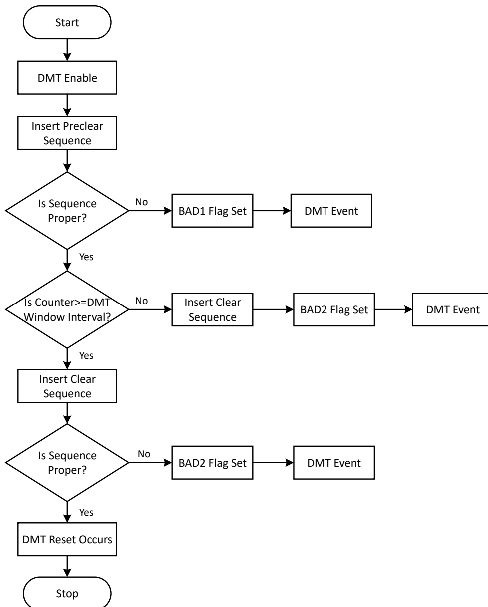
Figure 20-2. Flowchart for Clearing the DMT
