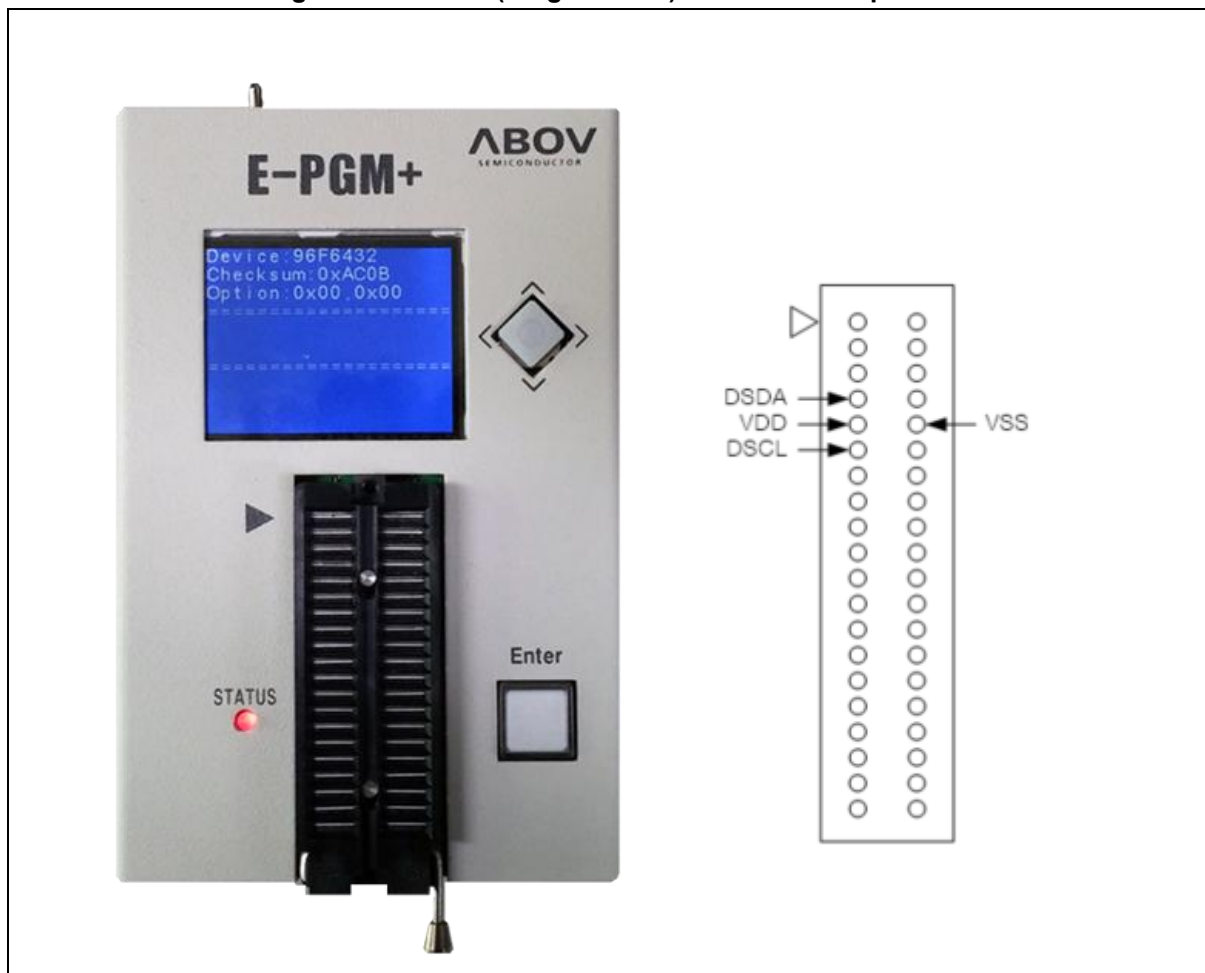
Figure 3. E-PGM+ (Single Writer) and Pin Descriptions
